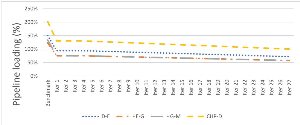
Figure 4. Level of congestion in several pipelines at hour 2613.
