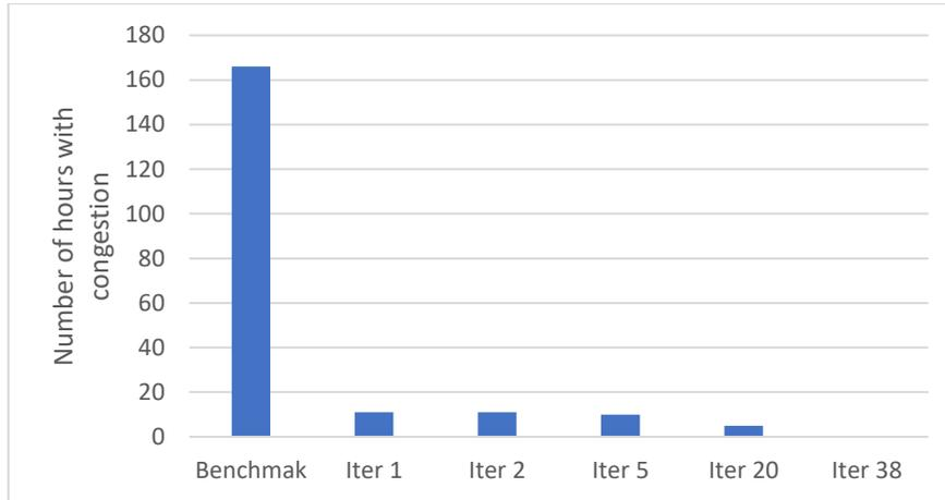
Figure 3. The number of network congested hours for the benchmark and iterative method (over iterations).
