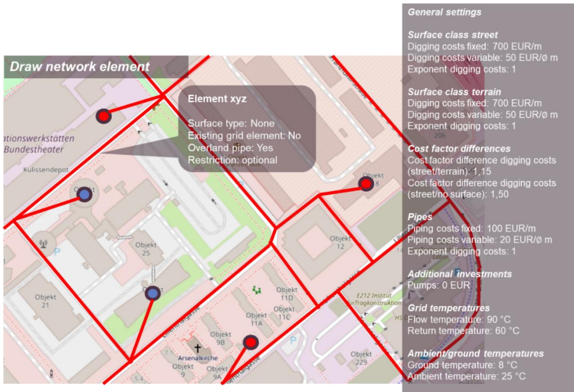
Figure 101: Setting overland pathway for pipes (mock-up).
